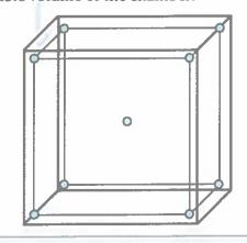
For Chambers up to 20 m³ (more than 2000 L): use 15 EDLMs (corners, center, wall centers) within the usable volume of the chamber.
